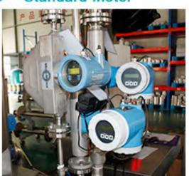
DN15-50 Gravimetric & Standard Meter Liquid Flow Meter Calibration Device
